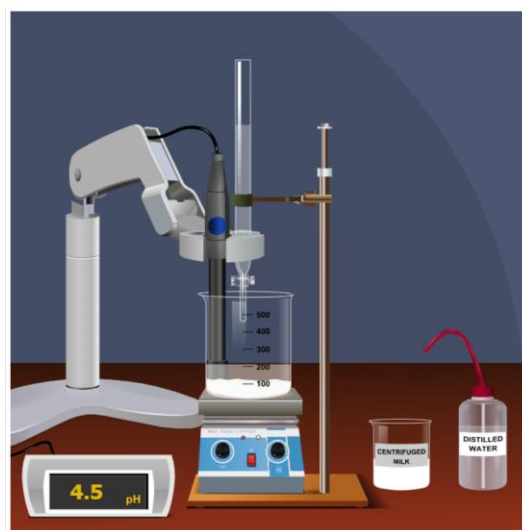
Isoelectric Precipitation of Proteins: Casein from Milk, Biotechnology
